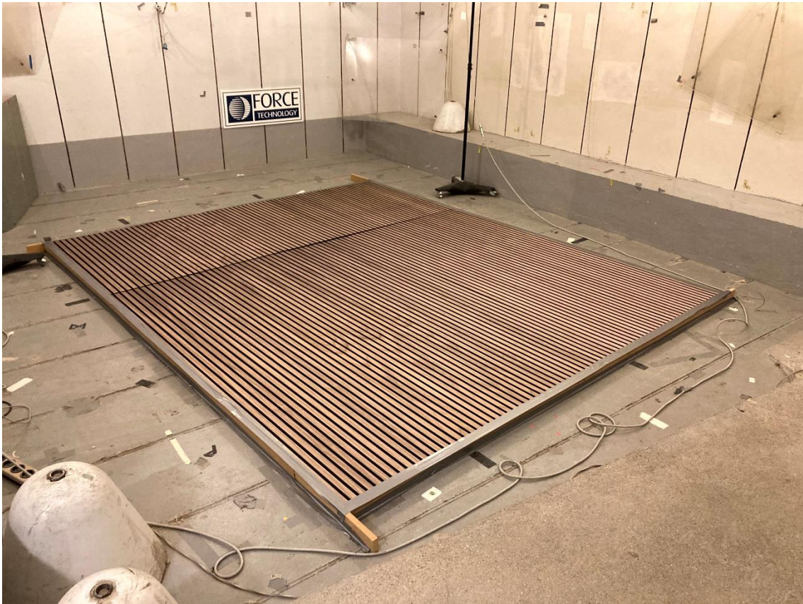
Figure 1 Acupanel Træ Panels mounted in the laboratory (Type E-65 mounting).
